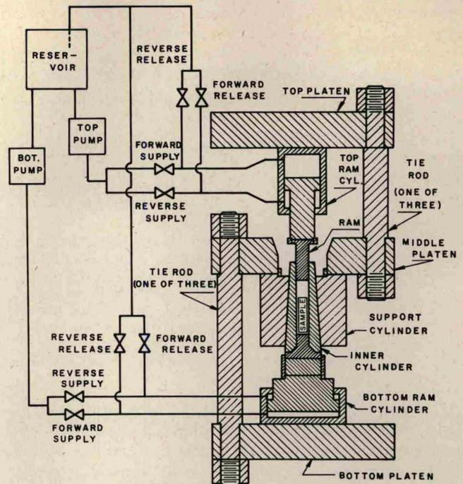
Fig. 1. Bridgman-Birch 30-kbar apparatus.
